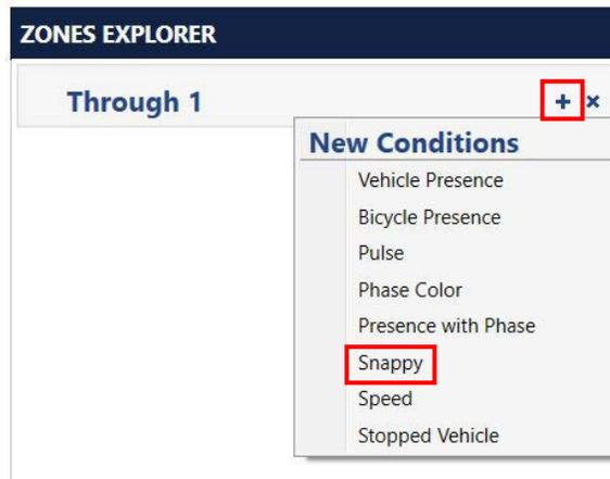
A Set Output action is automatically added to the Snappy condition.
