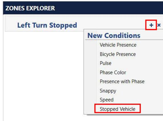
A Set Output action is automatically added to the Stopped Vehicle condition.
