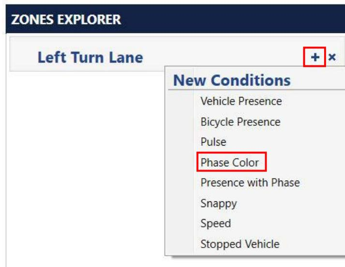
A Set Output action is automatically added to the Phase Color condition.
