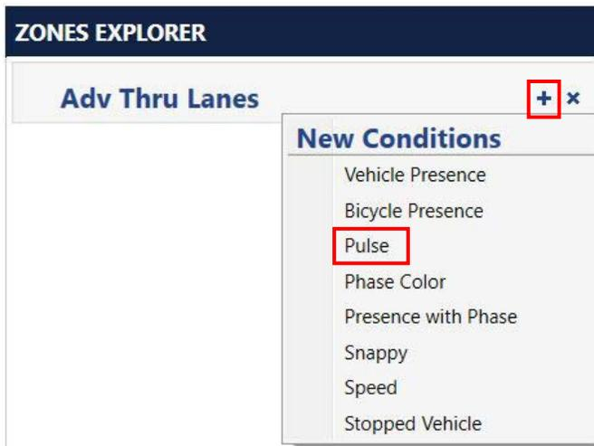
A Set Output action is automatically added to the Pulse condition.
