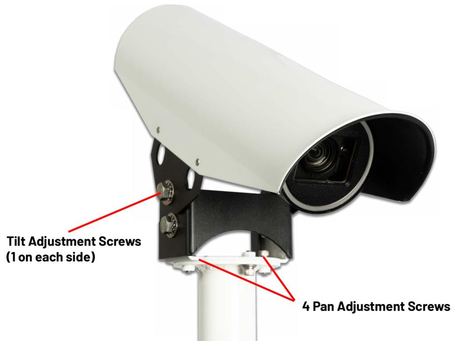
16. Pan the sensor left or right to center the image on the detection area, then tilt the sensor up or down to point the top of the camera just behind the stop line. This will typically provide a good field-of-view.
