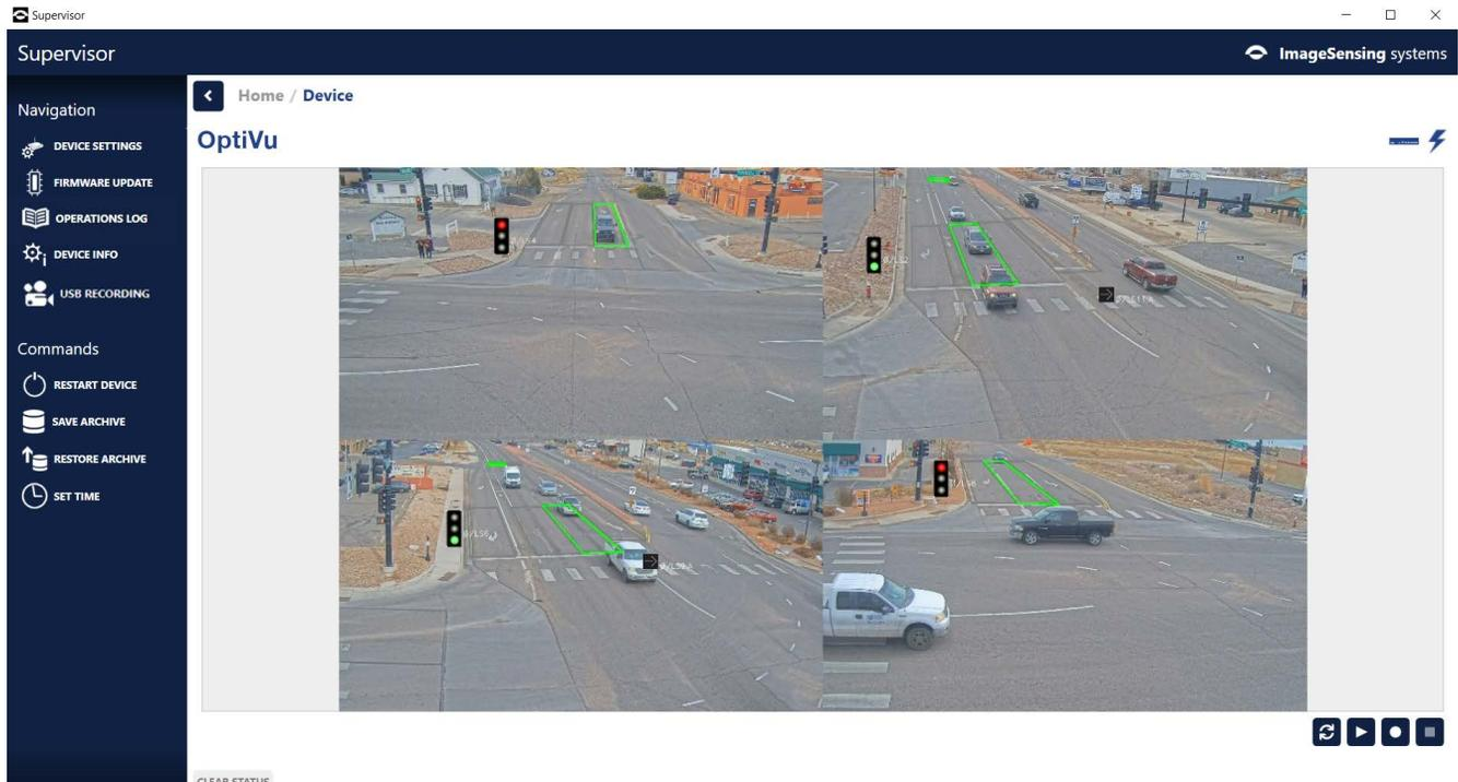
If cameras were already discovered, an image of all setup cameras will appear if the cameras are connected and online; one in each of the four quadrants of the image area. The order of appearance is determined by the order in which the cameras were added. The first camera will display in the upper left; second in upper right; third in lower left; fourth in lower right.
